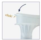
5 After all the liquid has gone down into the tube from the funnel, twist the empty funnel off the tube.
